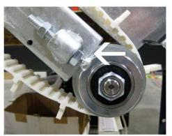
Configuration of nuts to make belt tight. Tighten the lower nuts in a way where the stretch pully is pushed in a downward incline.
