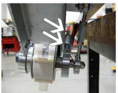
**Step 3:** The belt should be tightened so that there is approximately 2 inches from the center screw on the large guard to the inside of the belt, as it is being pulled in the opposite direction.
