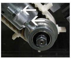
Notice with this side view, that there is the second set of nuts on the back side of the stretch pulley.
