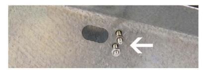
**Step 6:** Hold the Photo Eye in place as you screw it to the mounting plate and then finish the connection to the cable. **NOTE:** Only fasten the screws enough to secure the photo eye to the mounting plate, tightening too much will fracture the lens on the Photo Eye resulting in a failure to operate correctly.
