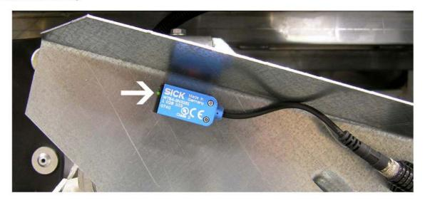
Step 2: To remove the Photo-Eye, first unscrew and pull apart the primary connection.
