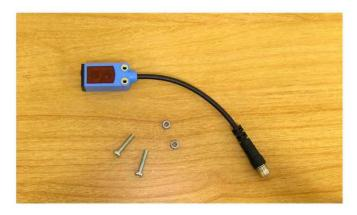
**Step 5:** When installing the new Photo Eye first insert the screws through the mounting plates cutouts for the screws; from the inside out. At this point, start threading the nuts as figured below.
