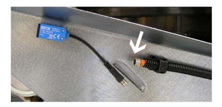
**Step 2:** Unscrew the two screws that hold the Photo-Eye in place which are located on the opposite side of the mounting plate.
