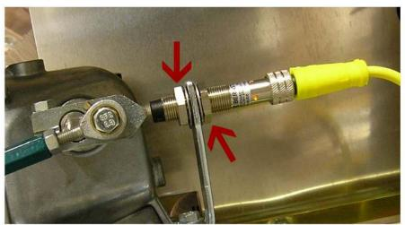
**Step 5:** The preferred distance between the Eccentric and the Magnetic Switch is 1/8th of an inch (figured below, left). Position of the eccentric after completing an entire revolution (figured below, right).
