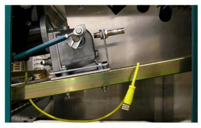
**Step 4:** You are able to loosen the nuts (figured below) to adjust the distance from the Magnetic Switch and the Eccentric. The prefered distance for best performance is 1/8th of an inch.
