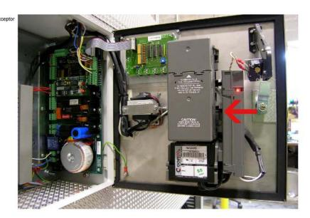
Step 2: To Remove the bill box, push the lock tab (below, left) forward on the top of the box and slide the box up (below, right)
