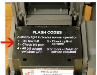
**Step 4:** To remove the bottom of the bill acceptor, look underneath as indicated below and depress the button while pulling the black "flash codes" box out away from the door
