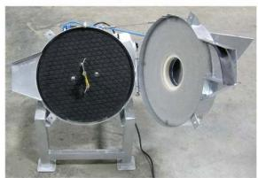
**Step 3:** With washer open (and hands away from the inside of the washer and all moving parts) turn on the washer to confirm that water is freely spraying through both water nozzles. The main brush nozzle (figured left) is more important and should be spraying substantially more than the pre-spray (figured right). If the path of water looks disturbed, unscrew nozzle with a 6mm Allen Key to clean.
